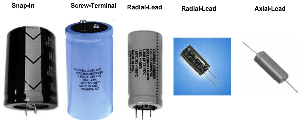
Figure 2.5: Package Options for Electrolytic Capacitors
