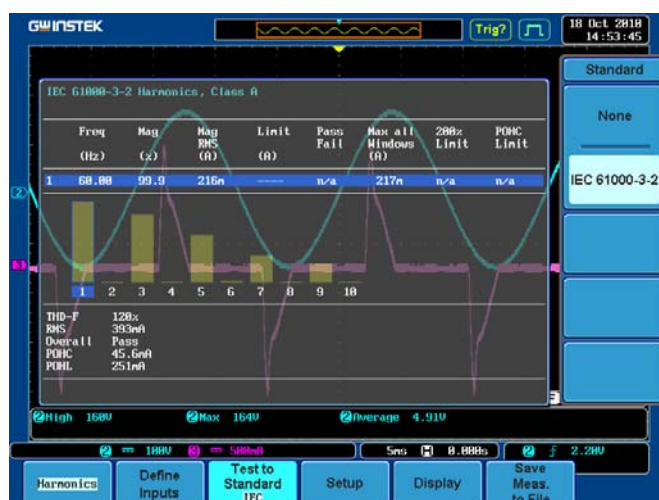
Figure 5: The GDS-3000 Harmonics function
